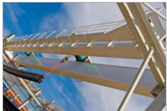
Double girder cranes 2x12t x 28m (Elastron S.A.)
