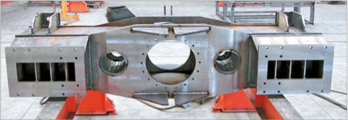
Strengthening plates (Gefyra Joint venture)
