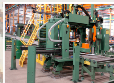
Thermal Cutting / Coping
