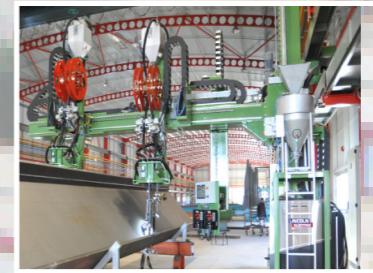
Welding Line for Box Girders & Beams
