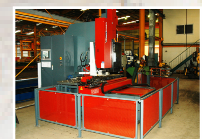
Plate Drilling & Punching Line
