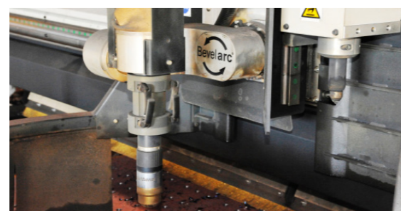
PLASMA & BEVEL ARC Plasma cutting with one or two heads and a bevel system for plate, pipe and profile bevelling.
