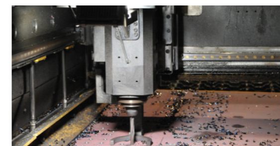
DRILTEC Drilling and tapping system with the option to automatically change tools.
